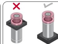
The body diameter (ØD) increases to the size of (ØPC). PC can be used with mounts C, but not with mounts type A.
