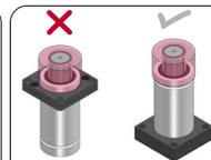
The body diameter (ØD) increases to the size of (ØPC). PC can be used with mounts C, but not with mounts type A.
